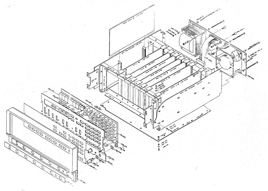
Figure 8-1. Model 8500 - Exploded View
