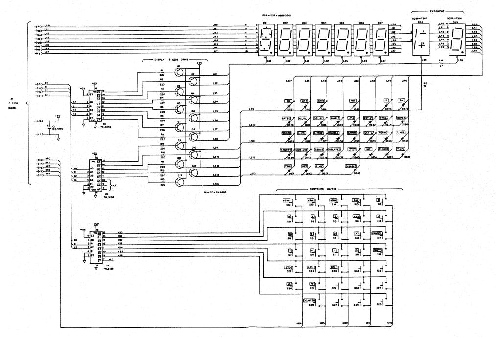
9-16 Display Board - Schematic Drawing
