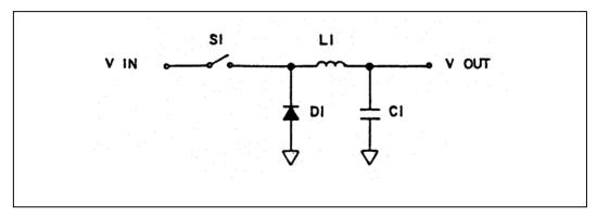
Figure 6-1. Switching Power Supply - Simplified Block Diagram
