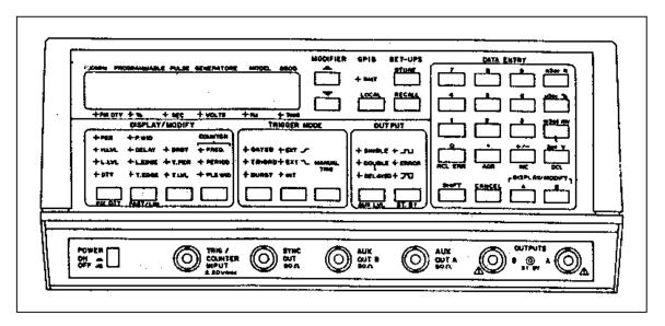
Figure 3-1. Front Panel Controls, Indicators and Connectors
