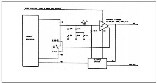
Figure 6-2. C.C.O & Clamping Circuit- Simplified Block Diagram
