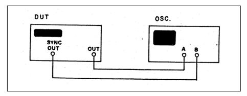
Figure 7-3. Systems Delay Adjustment.
