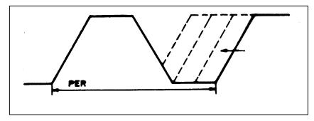
Figure 3-3. Output Wave Form With Error 4 (14)
