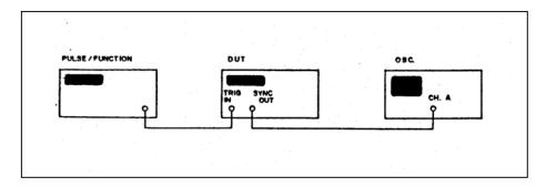
Figure 7-1. Trigger Input Sensitivity Adjustment.
